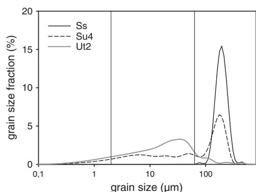
**Figure 2.** Characterization of soil types (sandy sand Ss, silt sand Su4, and clayey silt Ut2) used for the soil extraction experiment. The grain size distribution is described by plots of grain fraction (%) vs. grain size ( $\mu\text{m}$ ) of the substrate.
