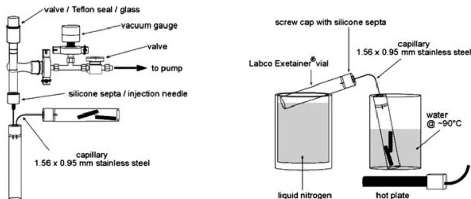
**Figure 1.** Schematic of the modified vacuum extraction method used for this study with an evacuation unit (left) and a cryogenic water trap (right). Exetainer vials with silicone septa and screw caps were connected with stainless steel tubing to extract water from soil and plant samples.
